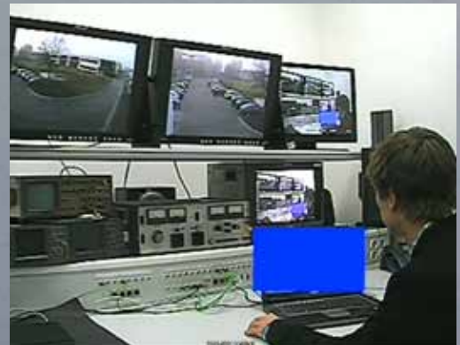
The screen of the laptop has been concealed while other image areas have been represented unchanged.
